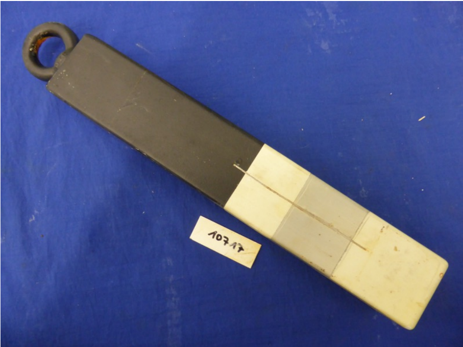
Picture 5 – Aluminium sample after 1000 h NSS exposure
