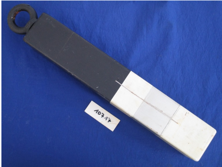
Picture 9 – Aluminium sample after 1500 h NSS exposure
