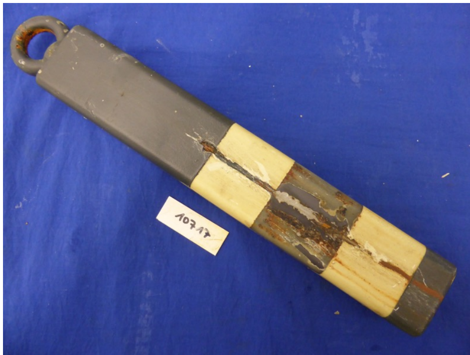
Picture 22 – Steel sample after 1000 h NSS exposure
