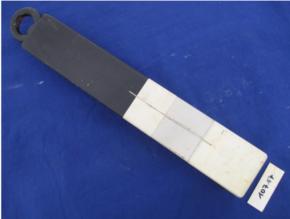
Picture 7 – Aluminium sample after 1240 h NSS exposure
