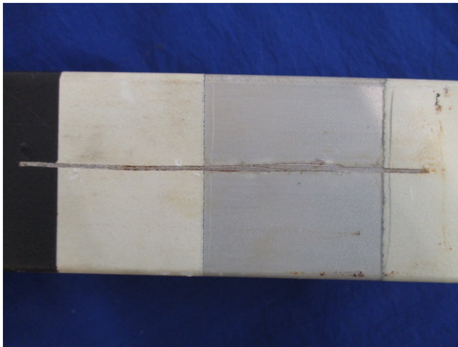
Picture 10 – Aluminium sample after 1500 h NSS exposure
