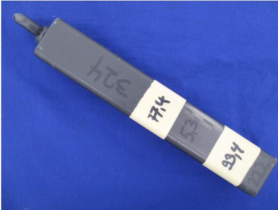
Picture 15 – Steel sample after 120 h NSS exposure
