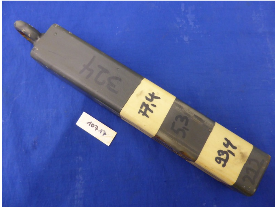
Picture 21 – Steel sample after 1000 h NSS exposure
