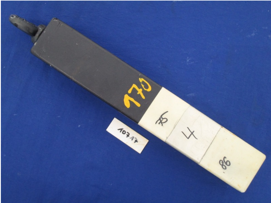
Picture 13 – Aluminium sample after 2000 h NSS exposure
