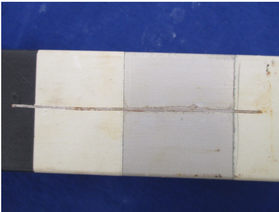
Picture 8 – Aluminium sample after 1240 h NSS exposure
